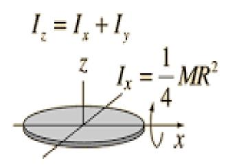
Since the x and y axes are identical by symmetry, they must have equal moments of inertia.
