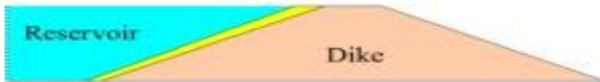
(c) Upstream surface protection
