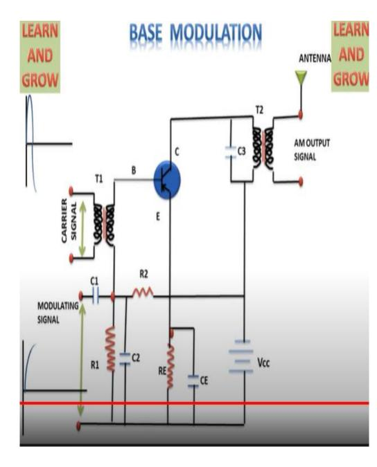
The circuit above uses capacitive coupling to inject the audio frequency signal [AF Input] into the Base of the transistor. The transistor circuit to the right represents another alternative. That circuit uses transformer couplings to inject the AF signal. Other than the method of coupling, the two circuits are basically identical
