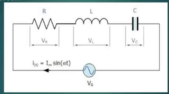
▶ The three basic passive components: resistance (R), inductance (L), and capacitance (C) have very different phase relationships to each other when connected to a sinusoidal AC supply.
